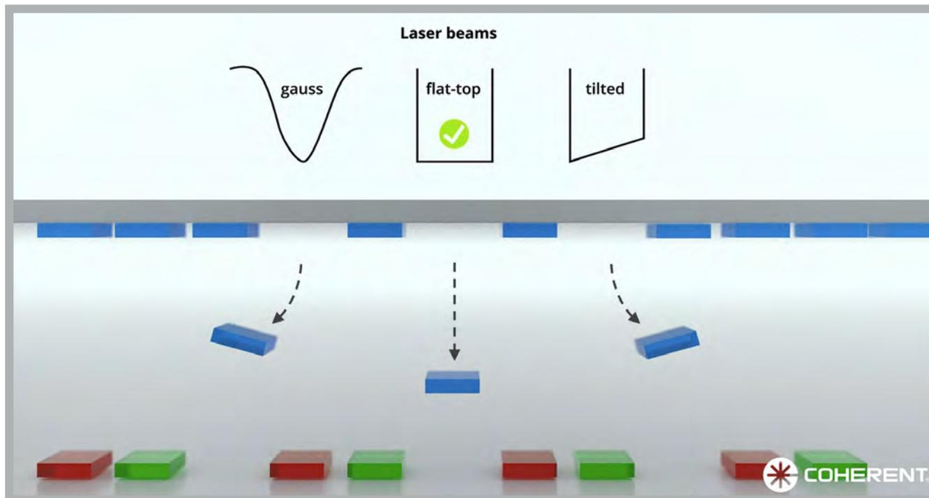
Figure 5: A highly uniform “flat top” beam profile is essential for accurate placement – not to scale.
